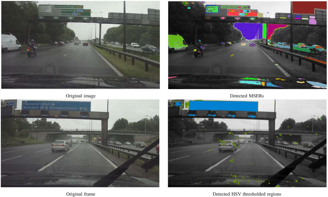
Fig. 6. Examples of MSERs and HSV-thresholded regions.
