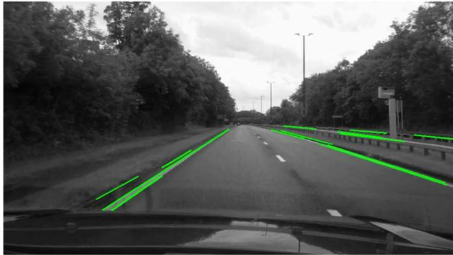
Reduced set of Hough lines and detected VP
